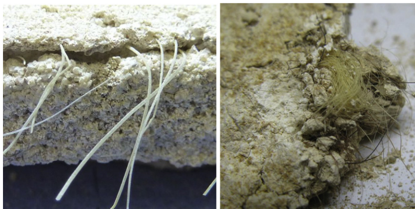
Fig. 1. Hair protruding from a modern failed plaster (left), and from 200-year-old chalk lime mortar (right). The hair from the modern samples was shown to be aligned, stiff and brittle. The sample being taken from new work in a private building in Somerset, England, in which a non-hydraulic lime putty plaster was reinforced with a hair imported from China, with failure of the plaster occurring due to the apparent partial digestion of the hair across the rivets resulting in detachment of the plaster from the walls; the historic hair sample was much softer and more randomly orientated, and was obtained from plaster removed from an early 19th century building on the South Coast of England.
