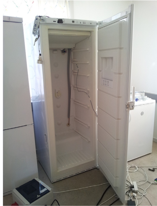
Fig. 1. The 333 liter domestic freezer used for the model identification and model predictive control (MPC) experiments.
