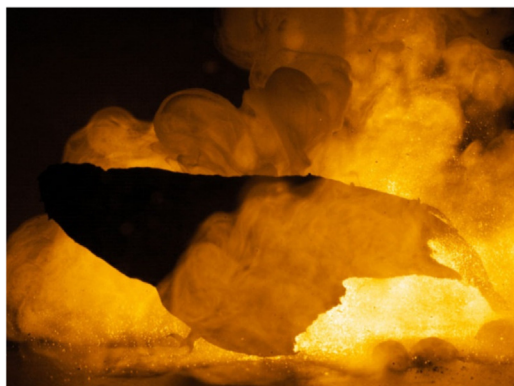
Fig. 1. High speed video image of the first moment of nanothermite foam combustion [11].
