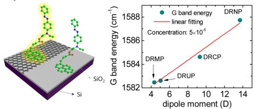
**The table of contents entry:** The Raman spectrum of chromophore/graphene hybrids with different dipole molecules has been investigated. It is shown that the graphene-enhanced Raman scattering (GERS) can be significantly changed by the dipole moment values. By the analysis of the Raman signals of graphene as well as the interfacial energy level match, a strong correlation between the GERS and graphene Fermi surface is revealed.
