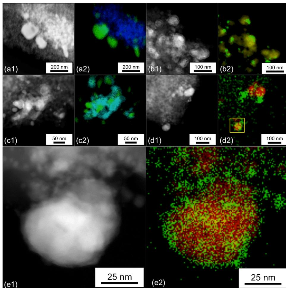
**Fig. 1.** HAADF-STEM image and EDX elements mapping of AgCo-GD (a1, a2), AgFe-GD (b1, b2), AgCu-GD (c1, c2) and AgNi-GD (d1, d2). (e1, e2) are enlarged images of yellow square of (d2). The green, blue, yellow, cyan, and red colors in EDX mapping correspond to Ag, Co, Fe, Cu, and Ni elements respectively. (For interpretation of the references to color in this figure legend, the reader is referred to the web version of this article.)
