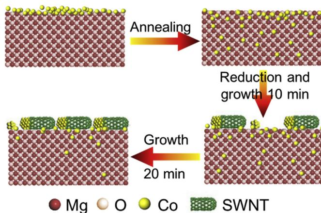
Fig. 1. Schematic illustration for the process of novel substrate-anchored solid solution catalysts preparation and high density SWNTs growth. (A colour version of this figure can be viewed online.)
