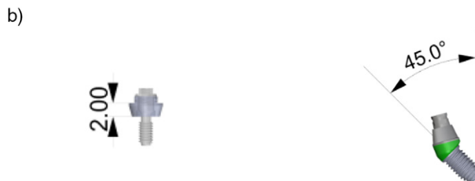
Fig. 2. Implant dimensions. An implant with an external hexagonal interface Titamax TI Cortical (Neodent®, Curitiba, Brasil) was used.
