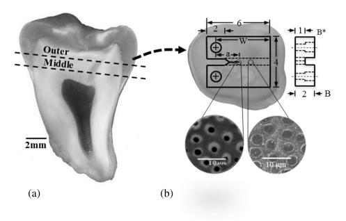
Fig. 1. Preparation of the compact tension (CT) specimens from sectioned human 3rd molars. (a) buccal-lingual section of a tooth showing the two coronal regions where the specimens were obtained (i.e. middle and outer regions); (b) view of a tooth section (perpendicular to its axis) and potential specimen. Note that in this orientation the crack will extend in-plane with the tubules, but perpendicular to their axes.
