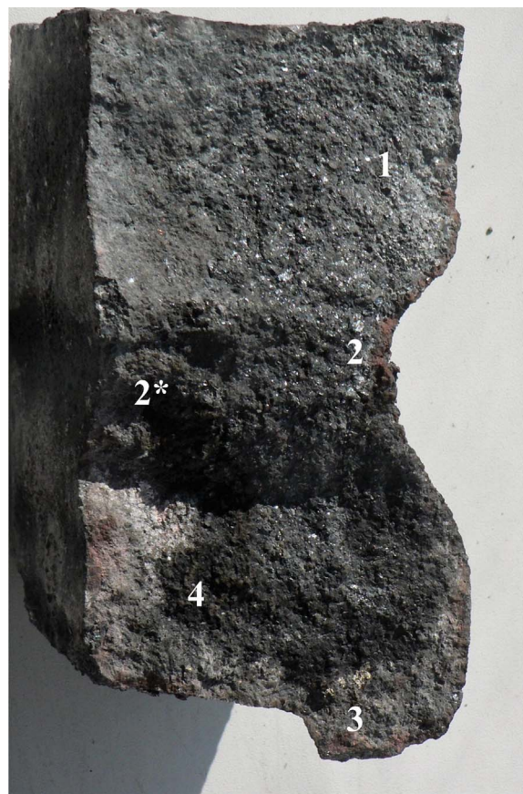
Fig. 3. The cross section of \text{Si}_3\text{N}_4 -SiC siphon block after testing.
