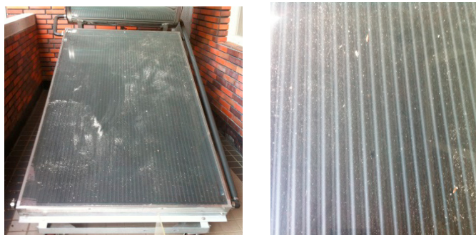
Fig. 1. The real model of a solar thermal heater (LHS) and dustfall on the flat-plate collector (RHS) for four months.
