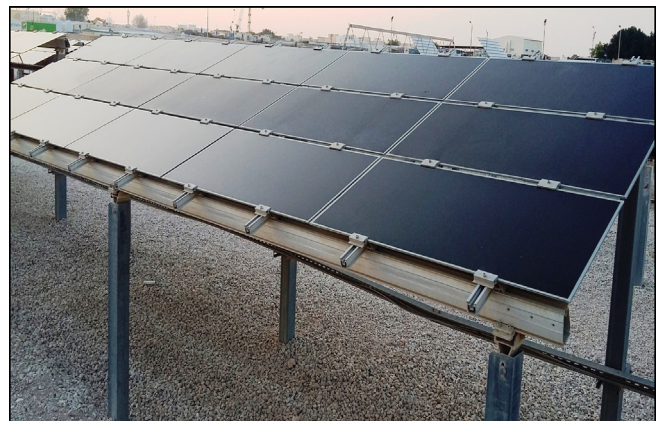
Fig. 1. Photo of a test PV array used in this study. The 12 panels on the outside (perimeter) were used for dust sample collection.
