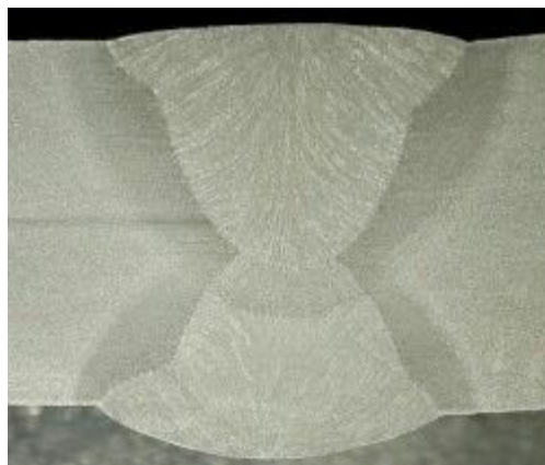
Fig. 1. Cross section of a multi-bead X-weld.
