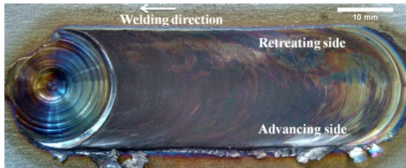
Fig. 1. The top surface of the weld accomplished at 1000 rpm and 50 mm/min.
