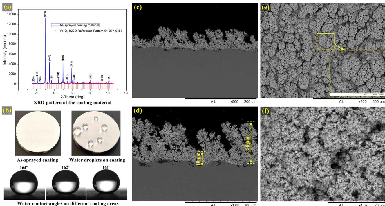
**Fig. 1.** (a) XRD pattern of the coating material; (b) Water droplets on the coating and WCA measurement; (c, d) Cross sectional microstructure; (e, f) Top surface microstructure.
