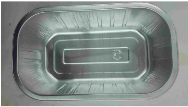
Fig. 1. An aluminium alloy 8006 "smooth-wall" container.
