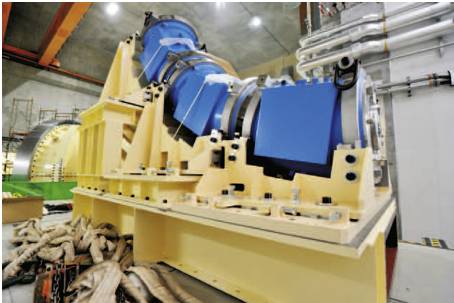
Fig. 2. Picture of the superconducting-magnet assembly for BM01-BM03.
