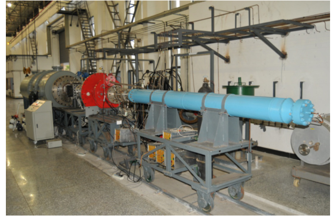
Fig. 1. Photo of the supersonic combustion facility in CARDC.
