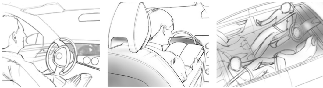
Fig. 1. Illustration of the three main scenarios for automated vehicles: From active driver to passive supervisor/passenger (left); Engagement in non-driving tasks (middle); Rearward facing seating arrangements (right).
