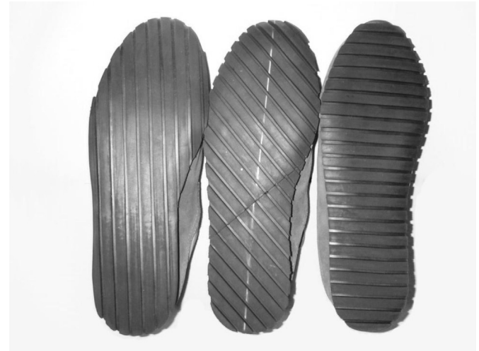
Fig. 2. Examples of study footwear. From left to right: parallel, oblique & perpendicular groove orientations. Each outsole depicted has 3 mm wide and 4 mm deep grooves.
