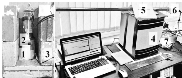
Fig. 1. On left: NaI spectrometer inside lead shield (front side of shield removed). 1) \phi 63 \times 63 mm NaI(Tl) scintillator, 2) R6091 PMT, 3) lead bricks. On right: NaI and ^3\text{He} neutron spectrometers during data acquisition. 4) Black box with NaI detector inside, 5) CHM-57 ^3\text{He} filled proportional counter, 6) ^3\text{He} neutron detector's preamplifier, 7) DT5780 Dual Digital Multi Channel Analyzer used to acquire data from both detectors.
