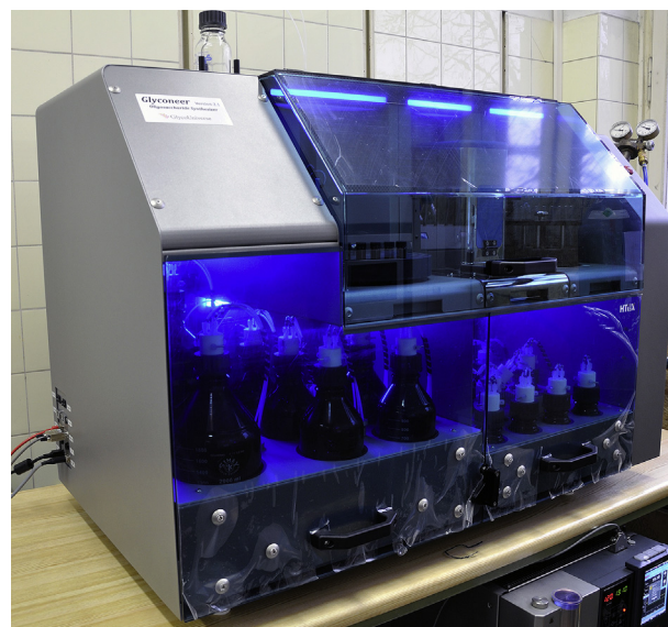
Fig. 2 The Glyconeer 2.1™—the first dedicated automated oligosaccharide synthesizer.
