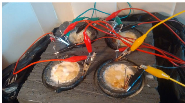
Fig. 2. Photo of one block with four aerobic bio-reactors each, in the process of recording electrical potential of the cells.
