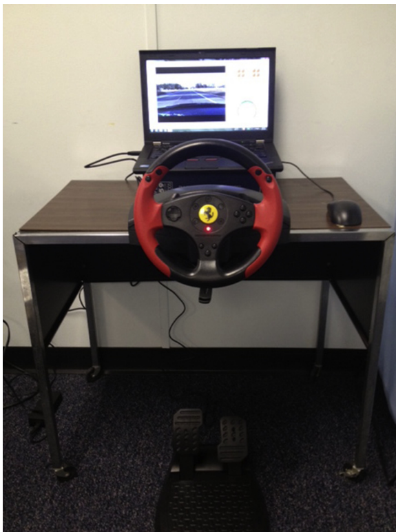
Fig. Driving simulator. The primary outcome measure of the present investigation was the mean brake response time using a computerized driving simulator. The brake response time was defined as the time from red light activation on the computer monitor while maintaining a constant accelerator speed to initiation of the brake pedal.
