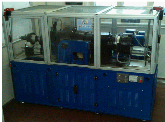
Fig. 2. Spline coupling test rig.
