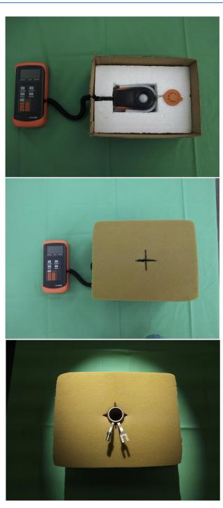
**Figure 1.** Experimental setting showing an isolated box with lux meter (SO 200K Sauter Light Meter) whose sensor was isolated and surrounded by foam material to reduce interference from other external light sources in the environment. In this example, we used a tube system with optical fibers.
