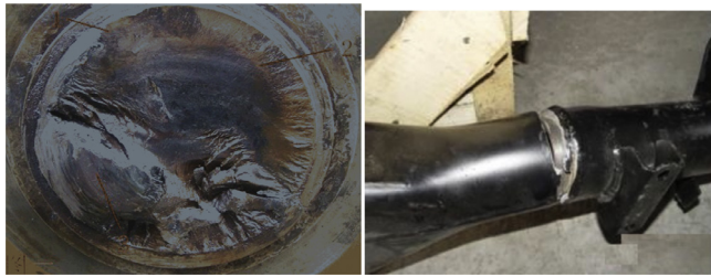
Fig. 1. Fatigue damage cases of axle.
