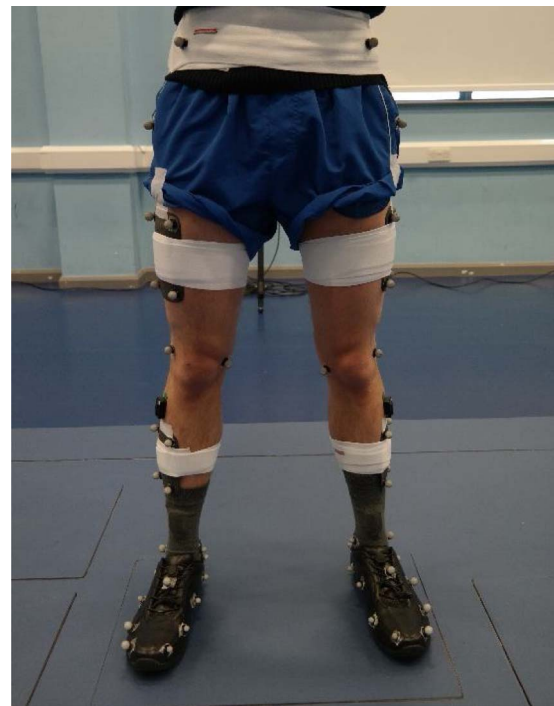
Fig. 1. Marker positions on lower limbs and pelvic during static calibration and walking trials.
