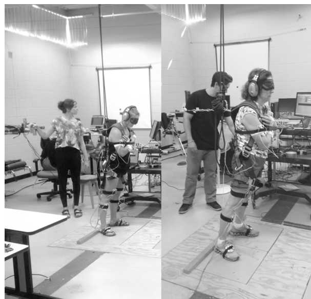
Fig. 1. Lean-and-release cable set-up for both younger and older adults. Participants were blindfolded and instructed to lean forward such that their body weight was supported by the cable from neutral stance. Perturbation onset time was calculated by a mounted load cell attached to the mechanical lift. Participants wore noise-cancelling headphones (Sennheiser PXE 450; 70 dB) while standing in a standardized foot position (heel centers 0.17 m apart, 14° between the long axes of the feet [26]). For each of the 110 trials (10 practice), participants judged whether the onset of the fall or a comparison sound (500 Hz 250 ms square wave burst; 77 dB) came first.
