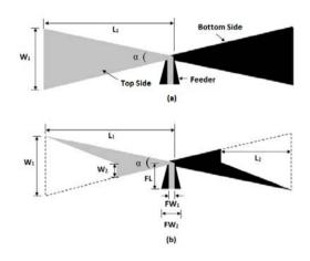
Fig 1. Geometry of the antenna configurations
