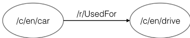
Fig. 1. Example of a single edge connecting two nodes. Symbols between slashes indicate the role and language of the respective items - 'c' stands for concept and 'r' for relation.
