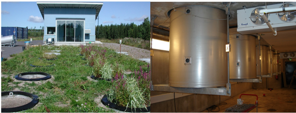
Fig. 1. The lysimeter facility in Lahti, southern Finland, with the eight lysimeters used in this study. The soil systems in the lysimeters were either vegetated or non-vegetated (left panel). The right panel illustrates the lysimeters as seen from below where each lysimeter rests on a set of three scales. The average mass of soil in a lysimeter was 2400 kg.
