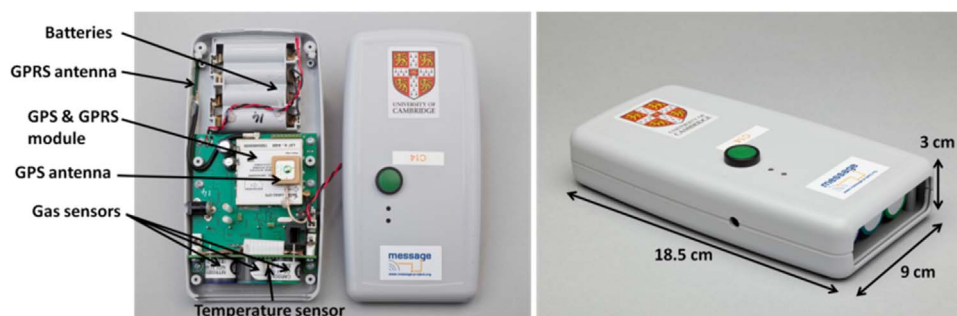
Fig. 1. Cambridge Personal Sensor (CamPerS) with essential components shown (approximate weight 450 g with batteries and 330 g without batteries).
