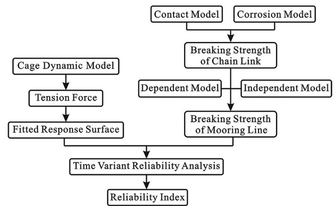
Fig. 1. The flow chart of the time variant reliability analysis model.
