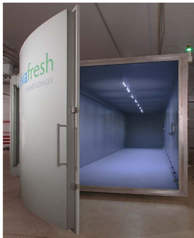
Fig. 2. Vivafresh 3332 ft 3 (94 m 3 ) hypobaric warehouse, installed in a 2 °C cold-room. Internal dimensions = 8.3 × 10 × 40 ft.
