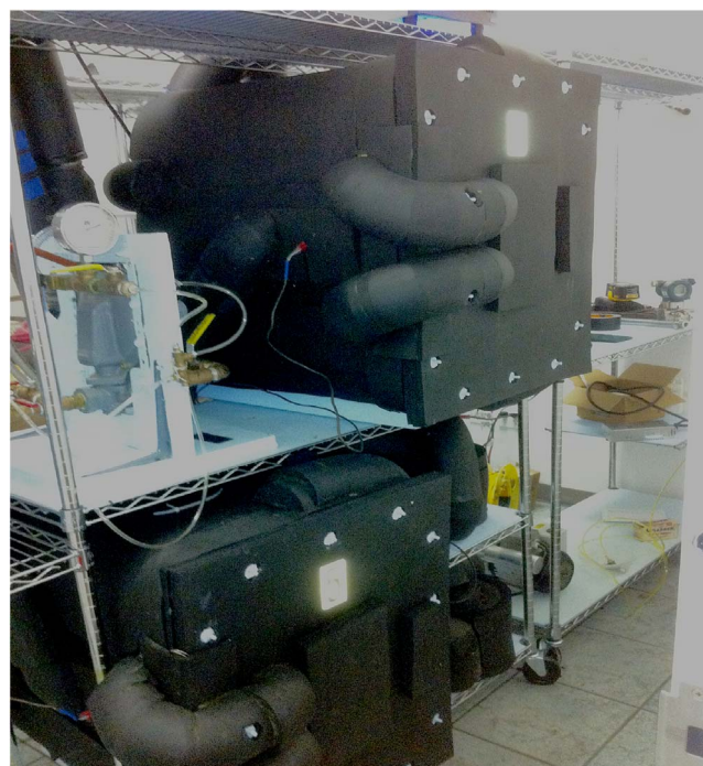
Fig. 1. Two VivaFresh 6 ft 3 (170 l) laboratory hypobaric chambers, installed in a 20–23 °C room.
