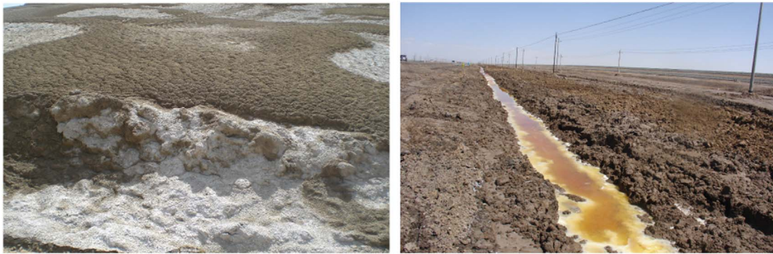
Fig. 1. View of a high salinity soil sampling site along the Golmud-Qarhan highway. Left: visible salt crystals (white); Right: salt precipitation in the roadside ditch along the highway.
