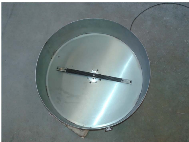
Fig. 2. Photograph of the centrifuge ice adhesion measurement system. The left end of the rotor shows the counterweight attached while the right end is the substrate on which ice is to be grown.
