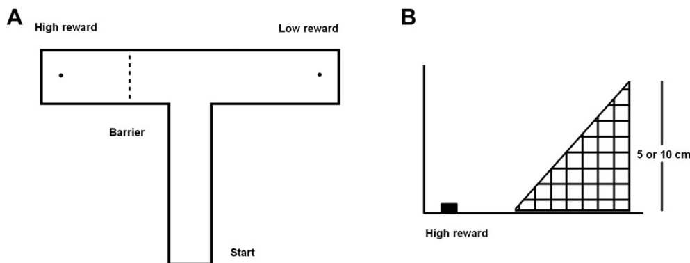
Fig. 1. Pictorial description of the apparatus used in the study. (A) A view from above of the high-walled T-maze used throughout testing, showing where the food rewards are located and where the barrier can be placed. (B) A side-view illustration of the barrier as it would appear in the arm of the T-maze. In order to obtain the reward, mice have to climb the vertical wall of the barrier and descend the slope on the other side.
