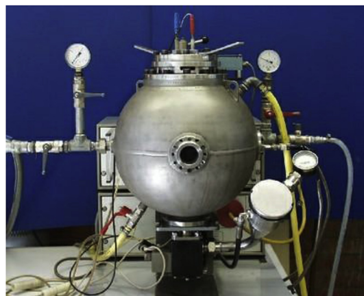
Fig. 1. 20 L sphere for the determination of the explosion indices P_{\text{max}} , K_{\text{St}} .
