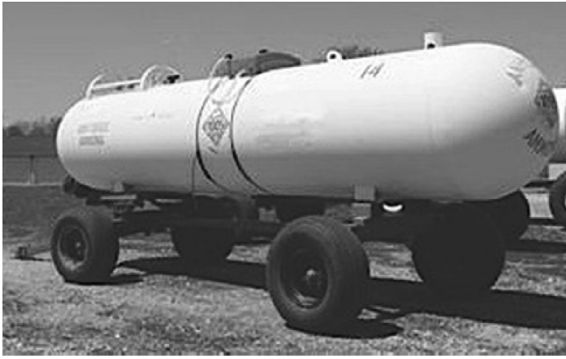
Fig. 1. Anhydrous ammonia nurse tank mounted on running gear. (Photo courtesy of the Federal Motor Carrier Safety Administration.)
