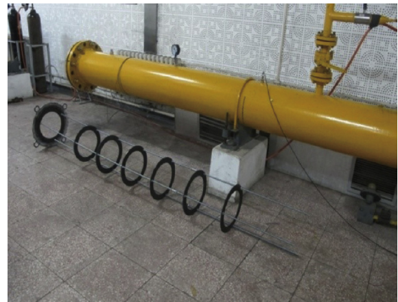
Fig. 2. Experimental duct and obstacles.
