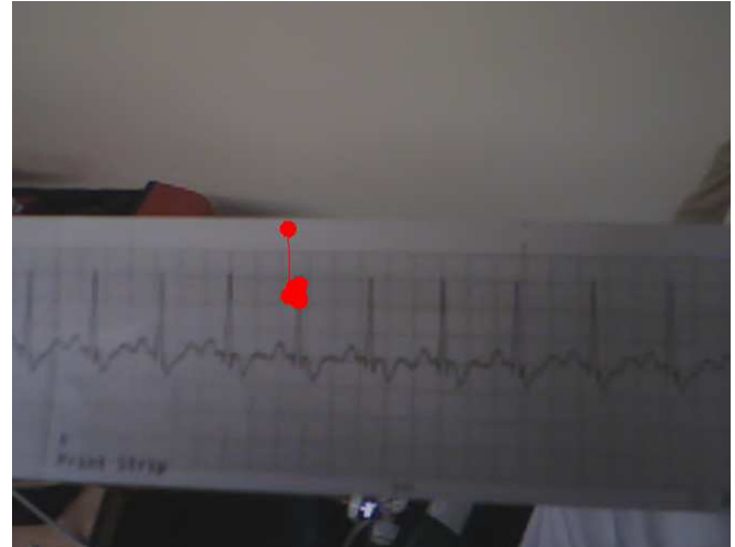
Fig. 3. The eye tracking video output. Note the pupil tracking (red) overlaid with the PoV capture.
