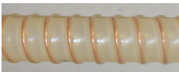
Fig. 2 – Example of a transfer hose with a metal spiral embedded in plastic wall.
