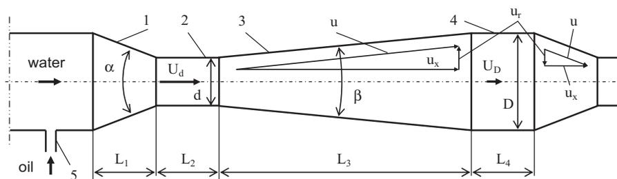
**Fig. 1 – Schematic of Venturi tube element of PFA with typical dimensions. 1 – confuser; 2 – neck; 3 – diffuser; 4 – wide part of apparatus; 5 – oil feed point (for first element of PFA only); u – flow velocity vector,  $u_r$  – radial velocity,  $u_x$  – axial velocity.**
