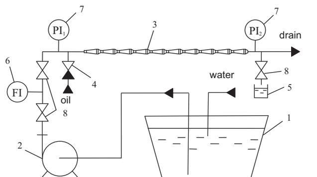
**Fig. 2 – Draft of experimental set-up for oil droplets dispersion in water in pulsating flow type apparatus. 1 – feeding tank; 2 – pump; 3 – PFA; 4 – non-return valve; 5 – container to collect samples; 6 – mass flow meter; 7 – pressure gauges; 8 – flow rate control valves.**
