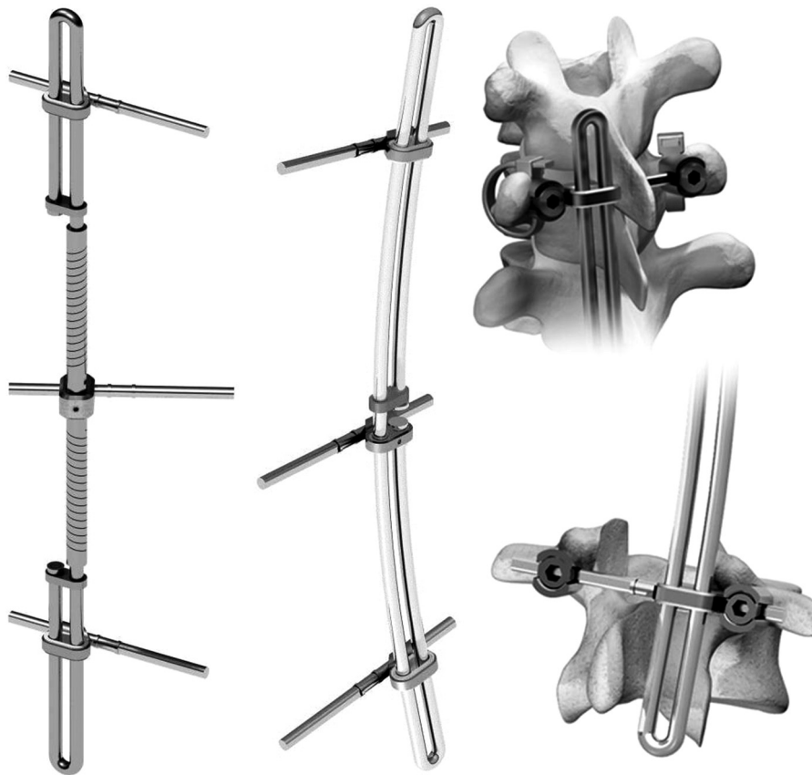
Fig. 1. The XSLATOR consists of two implants (Left and Center) that are posteriorly fixed to the vertebrae. The three bridges (Left and Center) can relatively slide axially, keeping the axial forces extremely low. The bridges are fixed to the spine using transverse process cables (XSFIX; Right Top) or two pedicle screws (Right Bottom).
