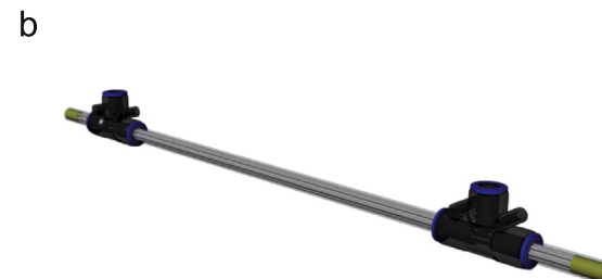
Fig. 2. Membrane module with 10 PES membranes. (a) Technical drawing of membrane module and (b) 3D drawing of membrane module.
