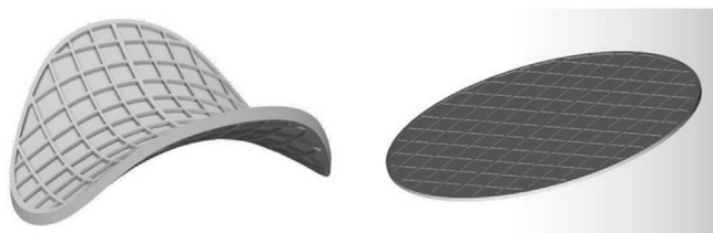
Fig. 1. Carriers used in the study; Z400 with 400 \mu\text{m} grid wall height (left), and Z50 with 50 \mu\text{m} grid wall height (right).
