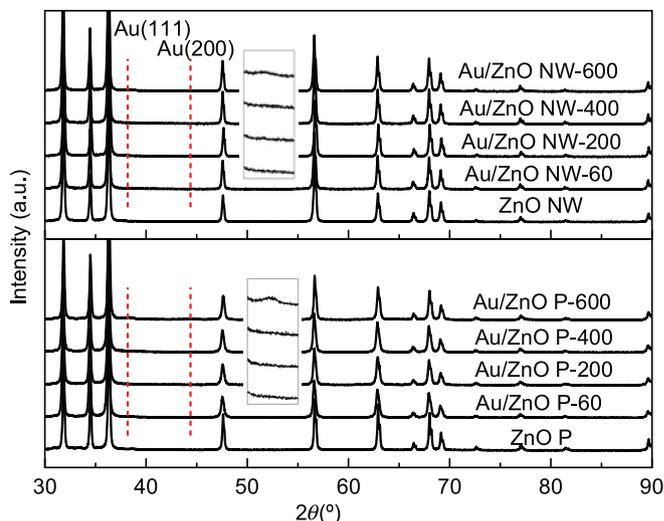
Fig. 2. XRD patterns of Au/ZnO NW and Au/ZnO P catalysts calcined at different temperatures. The insets show the enlargement of the Au (111) peak position.
