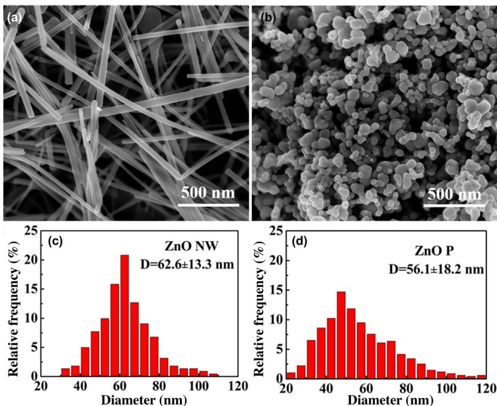
Fig. 1. SEM images and the diameter distributions of (a, c) ZnO NWs and (b, d) ZnO P.
