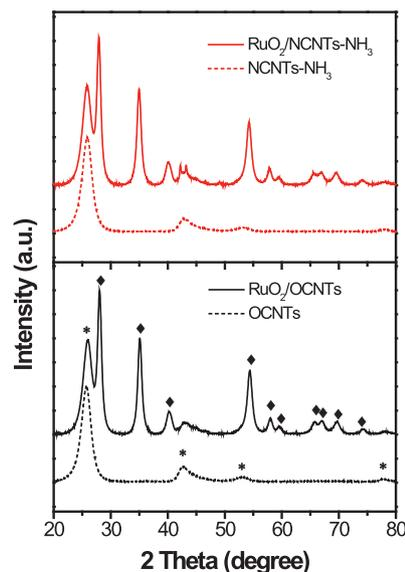
**Fig. 1.** XRD patterns of OCNTs, RuO<sub>2</sub>/OCNTs, NCNTs, and RuO<sub>2</sub>/NCNTs.
