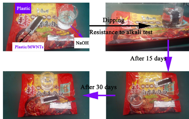
Fig. 2. Stability test of plastic/MWNTs in alkaline medium.
