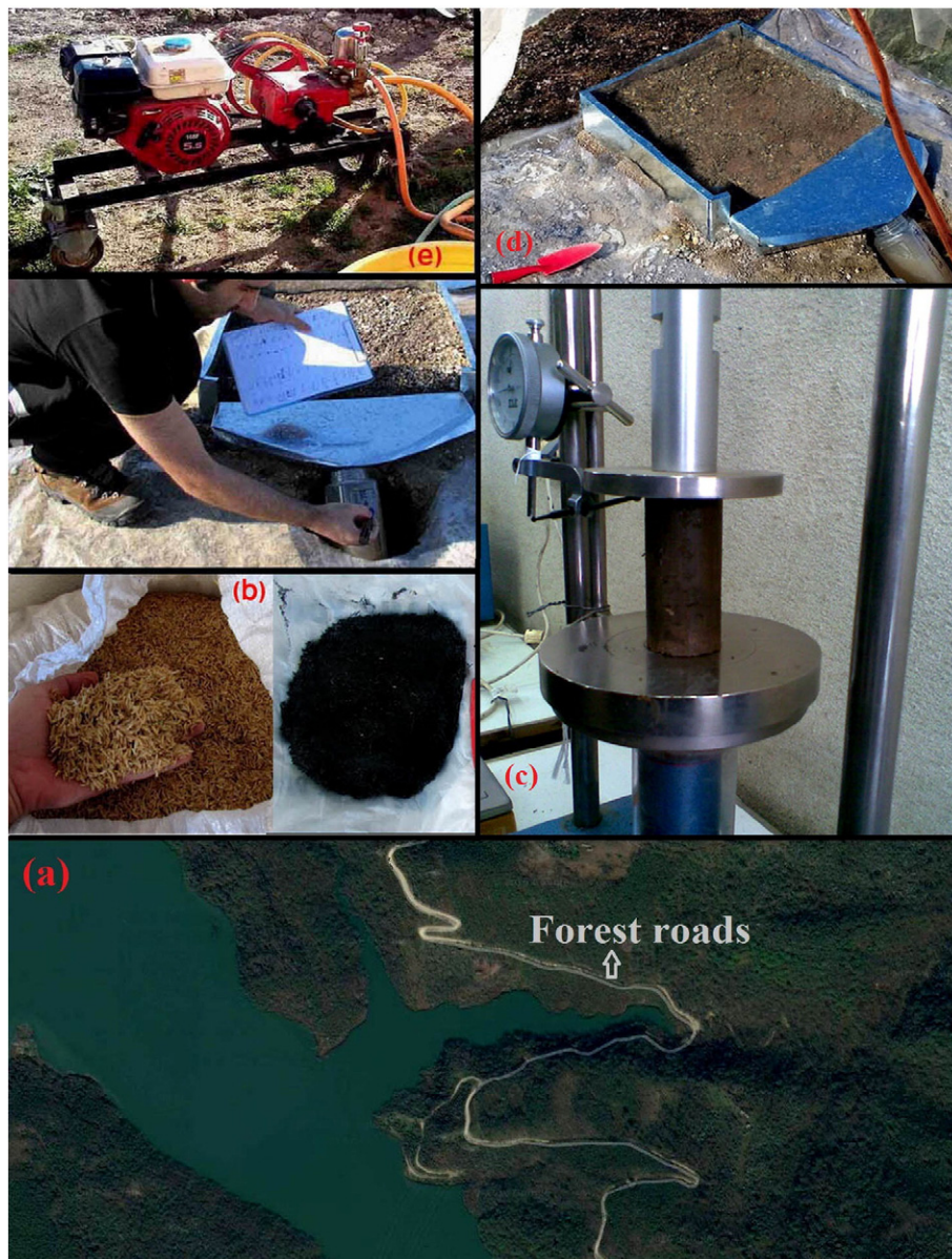
Fig. 1. Alborz earth dam and construction of forest roads in the Azarrod forest of Iran (a); produced RHA and rice husk (b); laboratory tests (unconfined compression apparatus (Afrazma)) to identify specification of different combinations (c); rainfall simulations to measure the runoff and soil loss (d) and use of mobile pump for field experiments (e).
